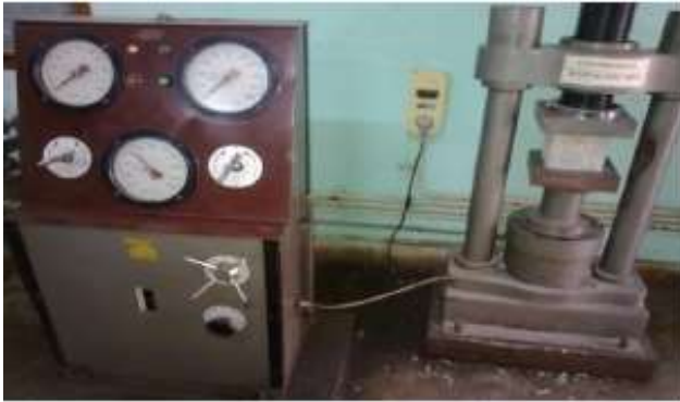
Fig 2. Compression Test on Concrete Cube
