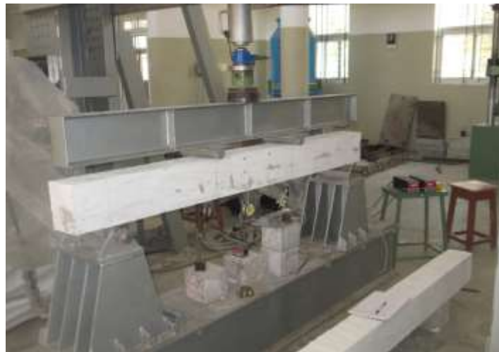
Fig 4. Testing of Beam Specimen
