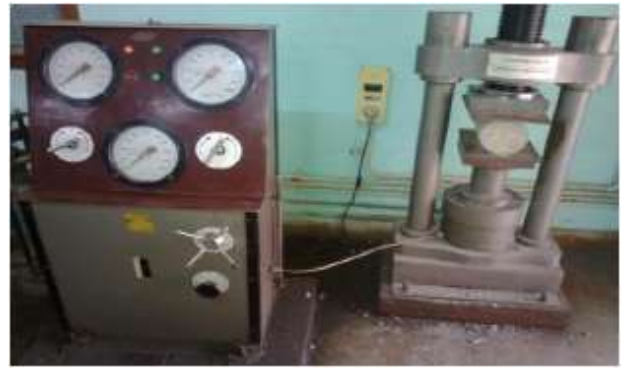
Fig 3. Split tensile Test on Concrete Cylinders
